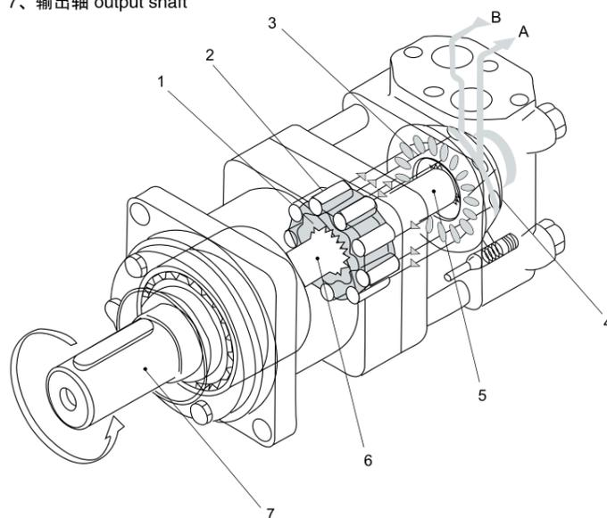
Shown as the drawing, high pressure oil goes into the motor's housing through the inlet, passing the auxiliary plate, distributor, then the working space between the orbit cam and rolls. Pressed by the high pressure oil, orbit cam rotates from the high pressure side to the low pressure side. The orbit cam makes rotation and revolution against the rolls, at the same time, high pressure oil is distributed continuously, thus, the output shaft can also rotate continuously.
